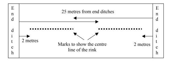
B.2.2 Marking 2 metres from each front ditch on the centre line of the rink
